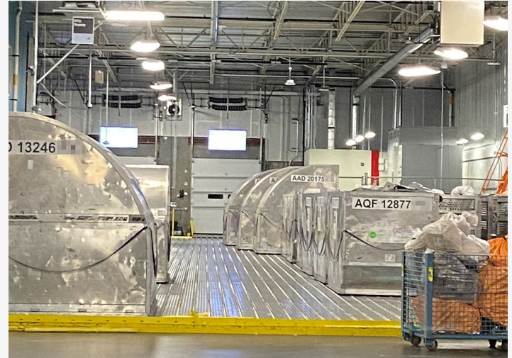
Staged Containers on Ball Decking
